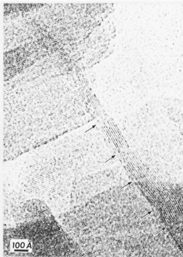
Figure 2. Image of normally sublimed (\text{AlPcF})_n crystallites showing the lengths of the unbroken lattices.
